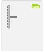
In areas with good signal strength, the antenna can be mounted within the VOLO cabinet. We recommend locating it away from the internal PSU to minimise any electrical noise interference.
